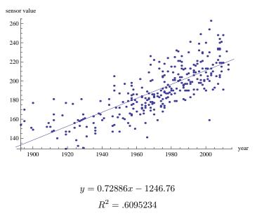
From this, we can calculate residuals for each point on the graph. Furthermore, by plotting the residuals at the value they correspond to, we can determine if patterns emerge, which would indicate that the linear model is an incorrect model.
