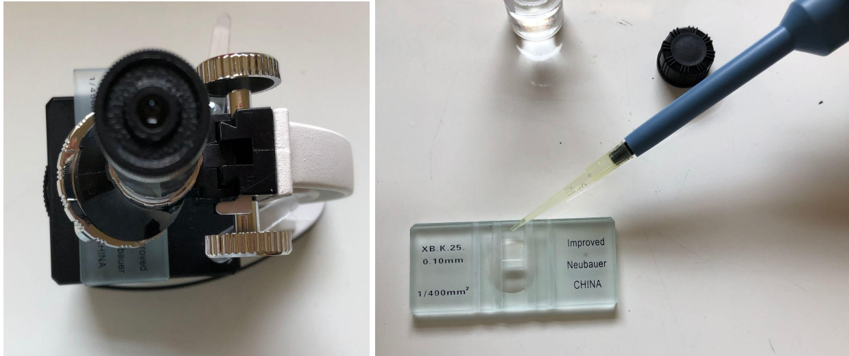
Figure 2. Set ups of the hemocytometer under the microscope and the OniLab microliter pipette filling the chamber.
