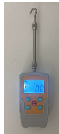
Figure 3: Photo of the Force Sensor used to measure the downward force in Newtons
